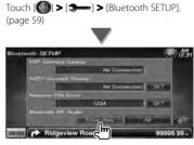
[Bluetooth HF/Audio] Sets the output speakers. ( Pront Only") "Front Only" : Outputs from the front speakers. "All" : Outputs from all the speakers.
